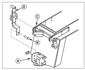
Figure 7. Rear Pulley Installation
